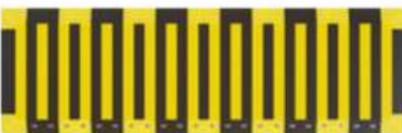
REVO SPEED HUMP R20 Length: 38 ft. x Width: 12 ft. x Height: 2.7 in. 22 CR51 ROAD STUDS CENTRAL POLYETHYLENE PLATES
