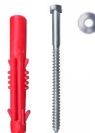
Anclaje en concreto Taquete "Extralarge" (3/4" x 14 cm) Tornillo "Ultrafix" (3/8" x 15 cm)
